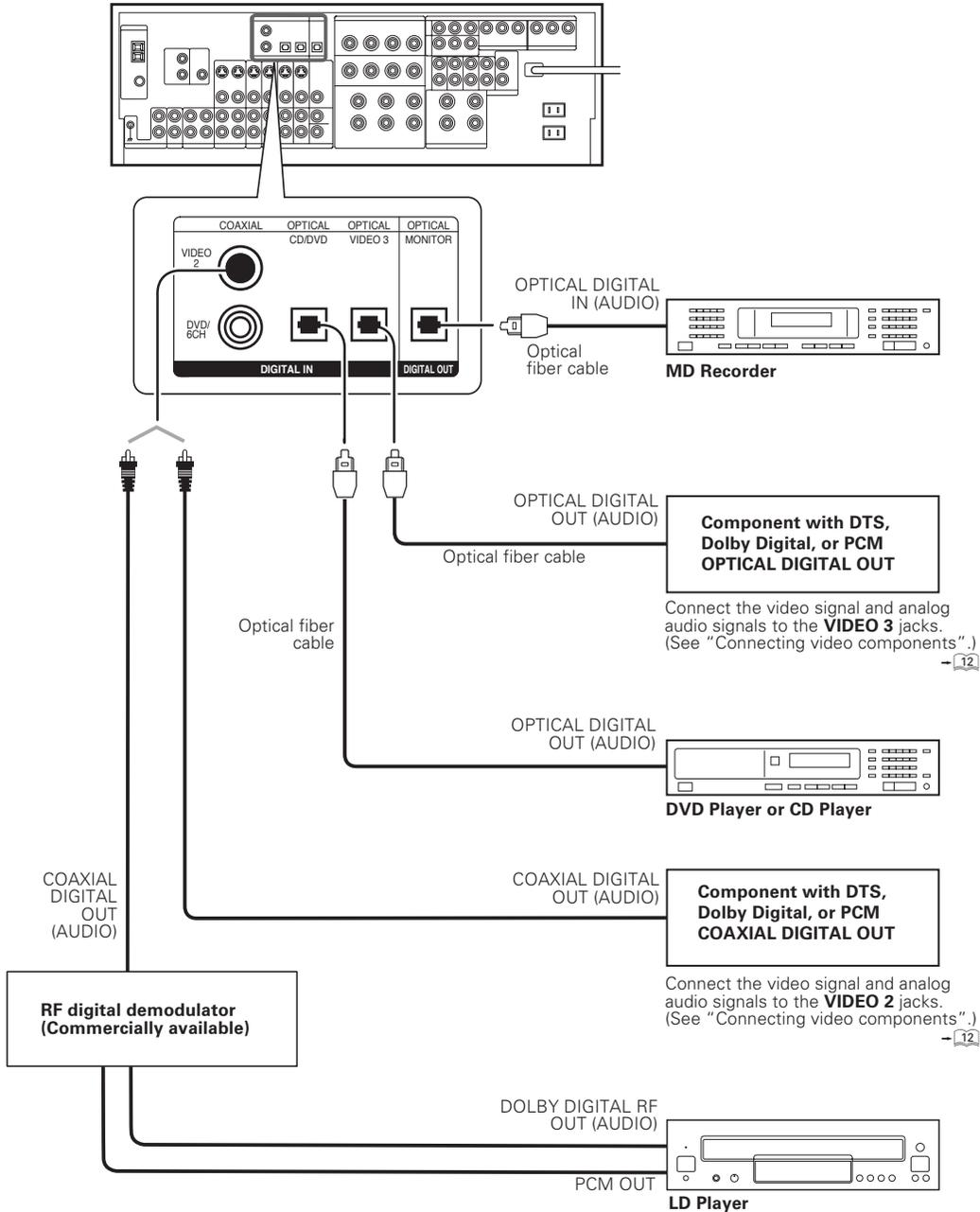
To connect an LD player with a **DIGITAL RF OUT**, connect the LD player to an RF digital demodulator (commercially available). Next, connect the **DIGITAL OUT** jack of the demodulator to the **DIGITAL IN** jack of the receiver. Connect the video signal and analog audio signals to the **VIDEO 2** or **VIDEO 3** jacks. (See "Connecting video components".)
