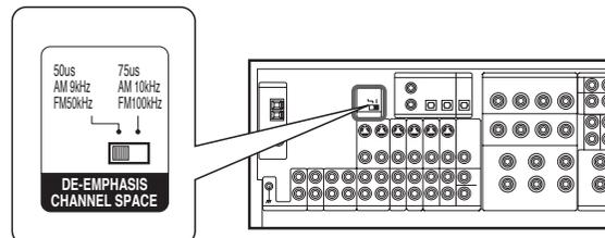
Turn the power OFF by pressing the POWER key before moving the switch level. Move the switch lever to match your area with a small screwdriver or other pointed tool, then turn the power ON again.
