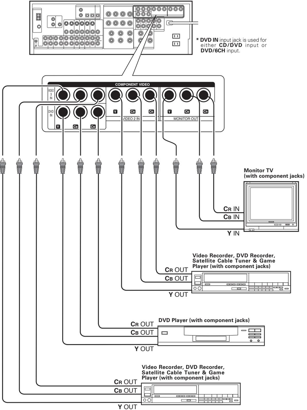
When connecting the TV to the COMPONENT jacks, be sure to connect all the other components to the COMPONENT jacks.
