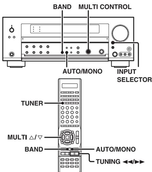
**1** Use the **INPUT SELECTOR** key or the **TUNER** key to select the tuner.
