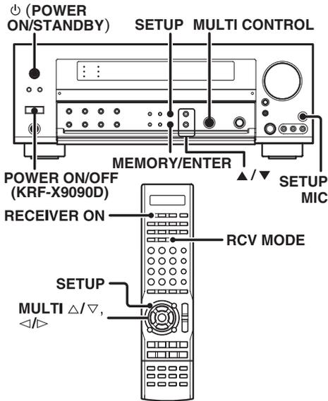
**1** When performing "Setting up the speakers automatically (AUTO SETUP)", connect the provided microphone for setup to the SETUP MIC jack.
