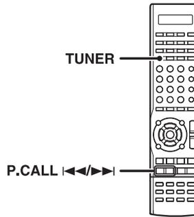
**1** Press the **TUNER** key to select the tuner as the source.
