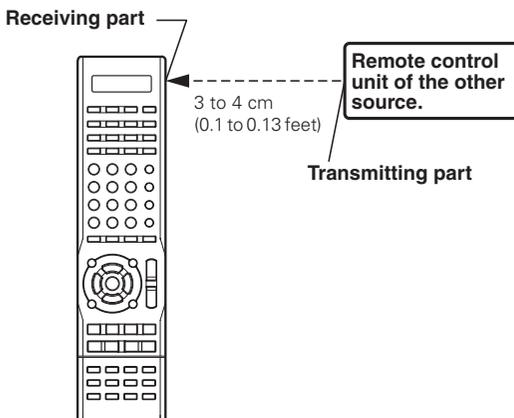
2 Press and hold the LEARN key for 3 seconds until blinks twice, then release the LEARN key.
