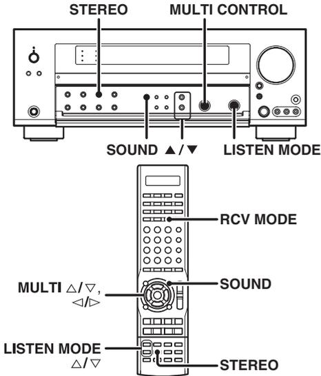
➊ For the remote control unit, press the RCV MODE key to switch to receiver mode.
