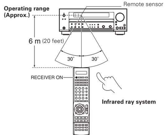
• When pressing more than one remote control key successively, press the keys securely by leaving an interval of 1 second or more between keys.
