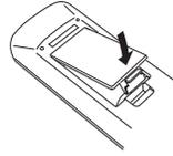
• Insert two AAA-size (R03) batteries as indicated by the polarity markings.
