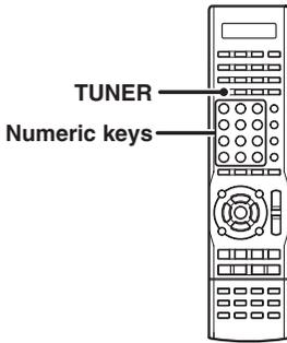
**1** Press the **TUNER** key to select tuner as the source.
